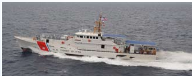
The Coast Guard Cutter Webber, the Coast Guard's first Sentinel Class patrol boat, arrives at Coast Guard Sector Miami Feb. 9, 2012. The 154-foot Webber is a Fast Response Cutter capable of independently deploying to conduct missions such as ports, waterways, and coastal security, fishery patrols, drug and illegal migrant law enforcement, search and rescue, and national defense along the Gulf of Mexico and throughout the Caribbean. U.S. Coast Guard photo by Petty Officer 1st Class Jennifer Johnson.
