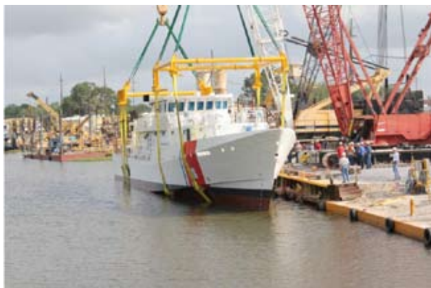
Coast Guard Cutter Bernard C. Webber settles into the water with the rigging attached. For the first part of the launch the cutter was kept rigged while the an inspection took place. If everything is satisfactory, the rigging is detached. USCG photo.
