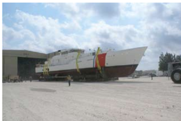
The total evolution to move Coast Guard Cutter Bernard C. Webber took three days. Here, Webber is shown on day one, exiting the fabrication shop on the way to the pier where the launch will occur. U.S. Coast Guard photo.
